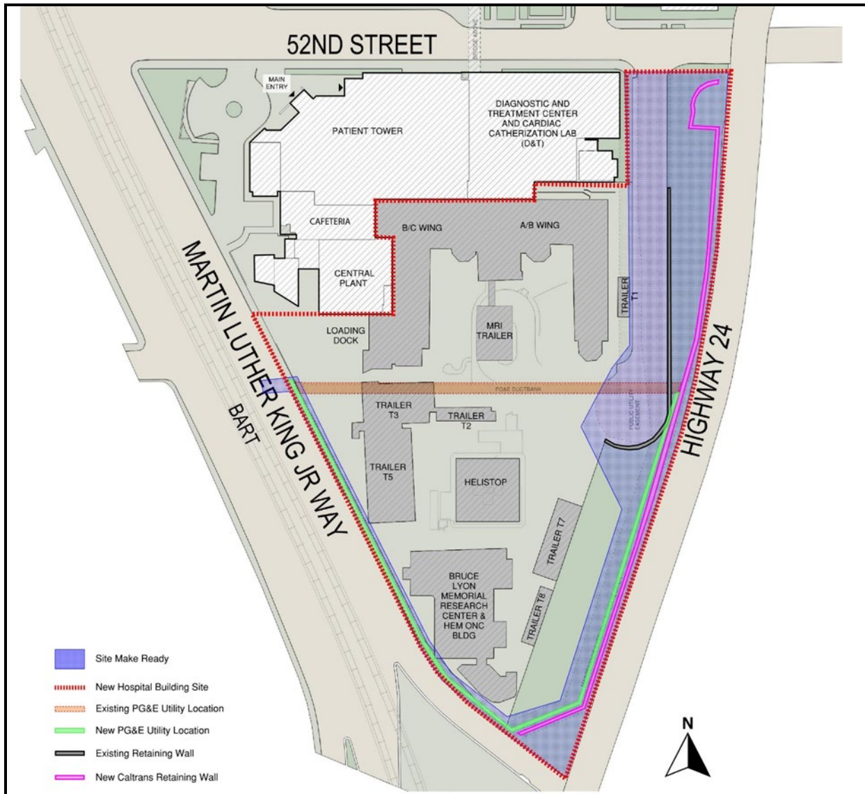
Figure 1: Caltrans Retaining Wall and PG&E Duct Relocation
